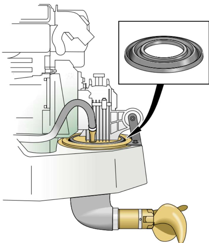
If you have an S-drive, the rubber seal between drive and engine bed has to be checked every year. If damaged, it must be replaced with a new seal immediately. Otherwise it should be changed every seventh year.
